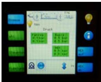
The touch-screen integrated into the control console, with many options for controlling the IBAK system components.
