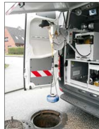
PANORAMO SI as pallet installation kit for the VW T5 (autarkic compact module) and as extension to an inspection system
