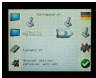
The touch-screen integrated into the control console, with many options for controlling the IBAK system components.
