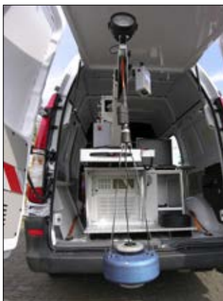
PANORAMO SI as pallet installation kit for the VW T5 (autarkic compact module) and as extension to an inspection system
