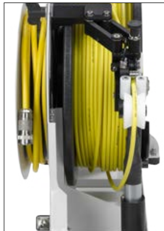
IBAK KT 180, adjustable cable guide for even cable winding
