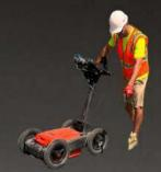
Ground Penetrating Radar is a non-destructive geophysical device used for subsurface exploration and operates by transmitting an electromagnetic pulse from an antenna into the ground and then capturing the partial reflections from subsurface layers. Any material with a different dielectric constant will either speed up or slow down the signal creating a hyperbolic trail. This is similar to a rock in a creek, the water bends around the rock leaving a tail wake.
